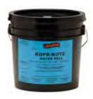
KOPR-KOTE contains copper flake, graphite, and rust and corrosion inhibitors in a water-resistant aluminum complex grease carrier. KOPR-KOTE is formulated to prevent excessive circumferential make-up and assure full hydraulic efficiency. KOPR-KOTE contains no lead, zinc, PTFE, or other materials that may be affected by elevated temperatures. KOPR-KOTE is unequalled in providing thread protection in demanding environments.
