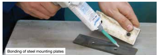
Bonding of steel mounting plates
