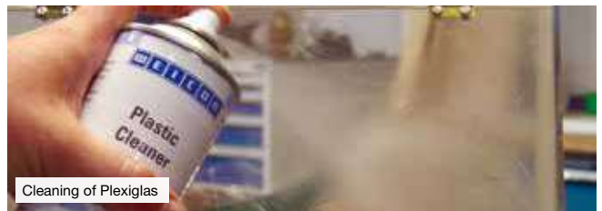
Cleaning of components before bonding
