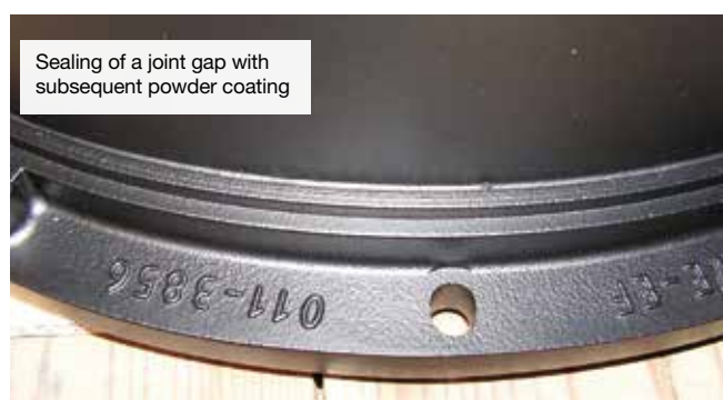
Sealing of a welding seam on a powder-coated rolling gate
