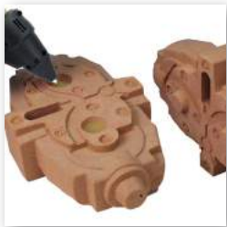
3 Assembly of sand cores for cylinder blocks.
