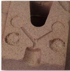
2 Sand cores showing recesses required for hotmelt.
