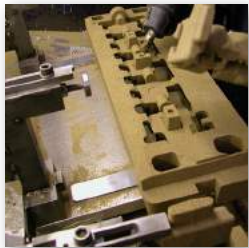
5 Typical cylinder head sand core assembly.
