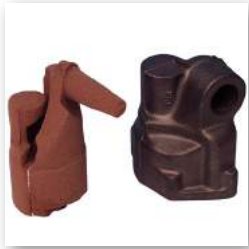
1 Internal sand core shape, and finished pump casting.
